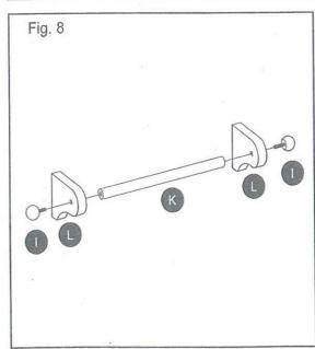
9. Insert wood dowels in the holes on the top side . push the bar to cart body using the bolt and washer to connect them.
